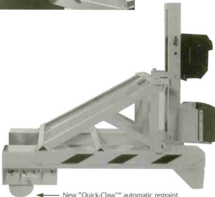
← New "Quick-Claw" ™ automatic restraint system locks attachment to forks automatically, eliminating the need for a safety chain to be applied by the forklift driver. Available as an option on any fork mounted DCM/DCMJ model.
